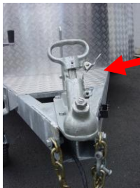
Coupling in UP position (ready for attaching onto the vehicle)
