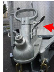
Coupling in Locked position (ready for towing)
